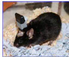
Fig-2. Freely behaving mouse undergoing EEG recording. Wireless EEG recordings (New Behaviour) Light weight: 3g (approximately 10% of the body weight) EEG recorder with built-in-accelerometer to record body movements.
