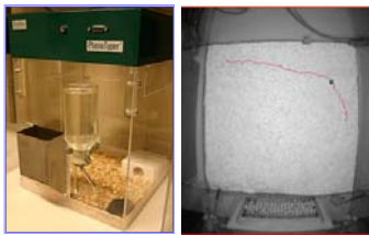
Fig-1. (A) PhenoTyper cage. (B) Videotracking with Ethovision. PhenoTyper cages: (30cm x 30cm x 35cm) with digital infrared sensitive video camera; Ethovision 3.0 (Tackxys, UK) was used as videotracking software. Activity (e.g. distance moved) and time spent in food and water zones can be assessed to compare the behavior of different groups of experimental animals.
